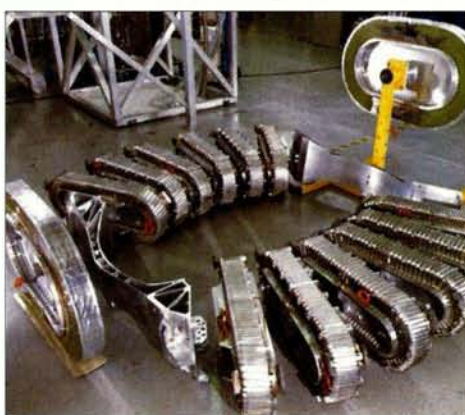
The 12 "racetrack" coils and two dipoles for the AMS superconducting magnet, built by Space Cryomagnets, UK, laid out in their approximate positions in the detector.
